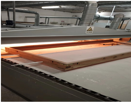
图2 快干抗黏连水性单组分清底漆应用实物图 Fig. 2 Real Application of Fast-drying Anti-sticking Waterborne Single-component Clear Primer
