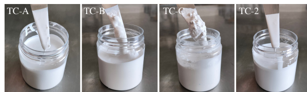
图3 在(35±2)℃条件下TC-A(7 d)、TC-B(2 d)、TC-C(1 d)和TC-2(60 d)贮存后的涂料外观 Fig. 3 Coatings Appearance of TC-A (7 d), TC-B (2 d), TC-C (1 d) and TC-2 (60 d) after Storage at (35±2)℃
